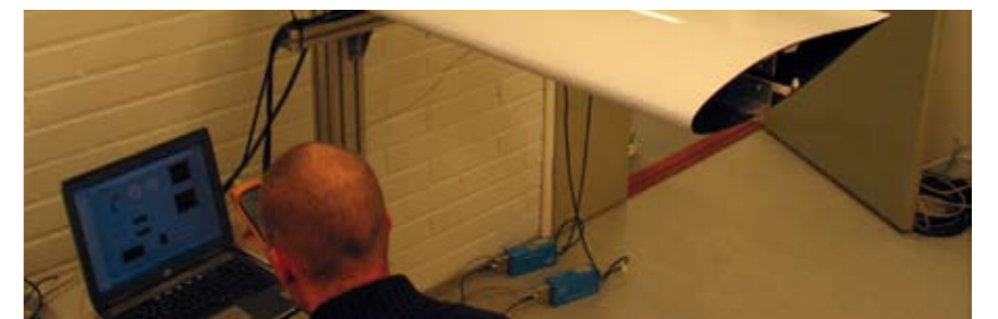
FE model and test set-up of an airfoil with embedded SMA wire actuated camber control.
