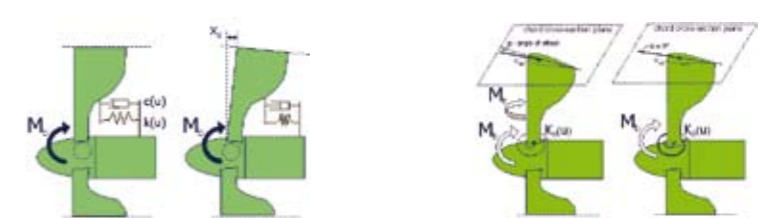
Active blade-hub interaction through tilting (left) or rotating the blade (right). With the second, rotating is done around the longitudinal axis of the blade, changing the angle of attack. In both cases the stiffness of the interface is controlled.
