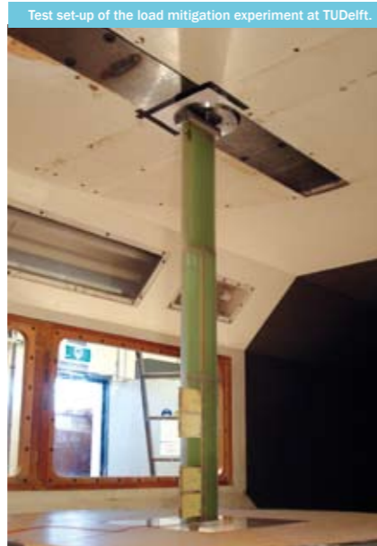
Test set-up of the load mitigation experiment at TUDelft.
