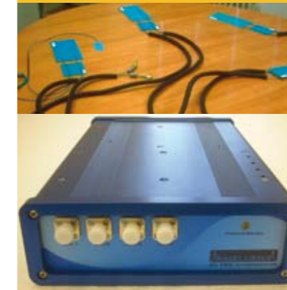
Figure 6: FBG sensor patches and 4channel interrogation unit to be installed in the test wind turbine.
