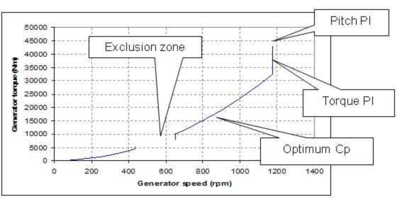
This is the torquespeed curve, showing the exclusion zone for avoiding tower excitation caused by the blade passing frequency coinciding with the first tower mode.
