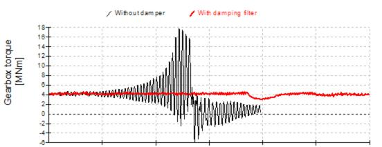
Without a drive train damper, the drive train would be completely unstable at some wind speeds.
