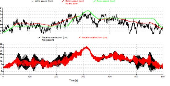
This simulation demonstrates the beneficial effect of the speed exclusion zone. Deviations from optimum Cp result in a small loss of energy.
