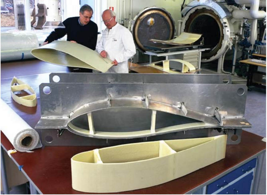
Figure 16 Thermoplastic composite rotorblade sections manufactured in a one-shot vacuum consolidation technique using the aluminum mold shown in the middle (92).
