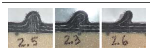
Figure 7. Sections through wrinkle defects of differing depths in a sandwich face laminate. The face laminate thickness is ~5.4 mm in each of the cases shown.
