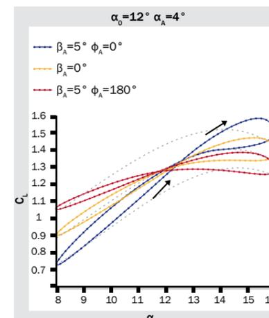
Figure 3: Dynamic stall loops for a pitching airfoil with a cyclic trailing edge deflection.
