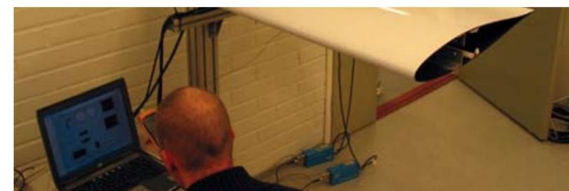
FE model and test set-up of an airfoil with embedded SMA wire actuated camber control.
