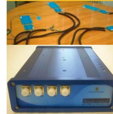
Figure 7: A photograph of a blue 4-channel FBG interrogation unit.
