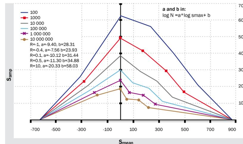
Figure 1: Constant Life Diagram for MD material.
