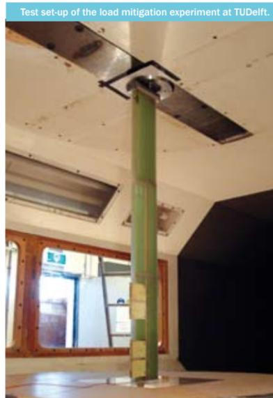
Models able to evaluate the potential for load reduction in smart rotor control have been developed. The aero-servo-elastic model, which was developed, serves as a prediction tool, but also as a controller design platform.
