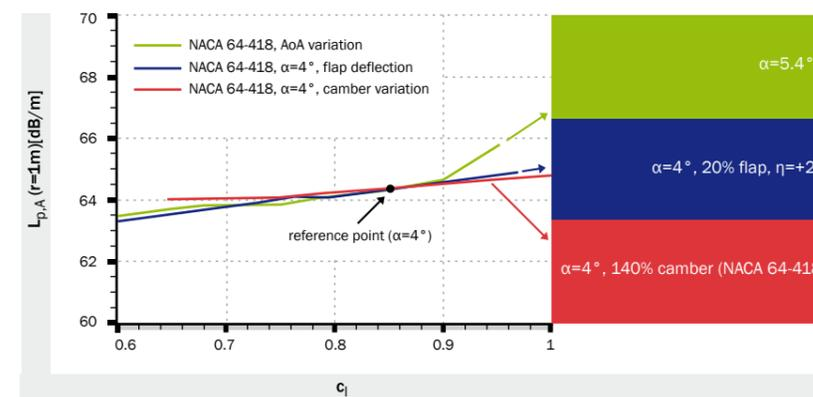
Noise generated by a baseline, a discretely rotated flap and a continuously deformable trailing edge flap (camber variation).
