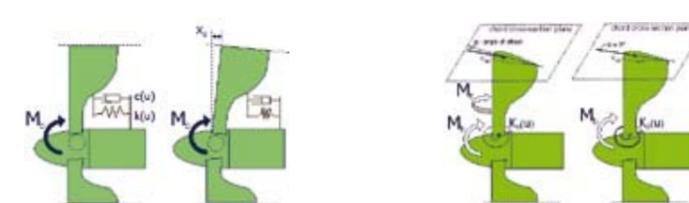
Active blade-hub interaction through tilting (left) or rotating the blade (right). With the second, rotating is done around the longitudinal axis of the blade, changing the angle of attack. In both cases the stiffness of the interface is controlled.
