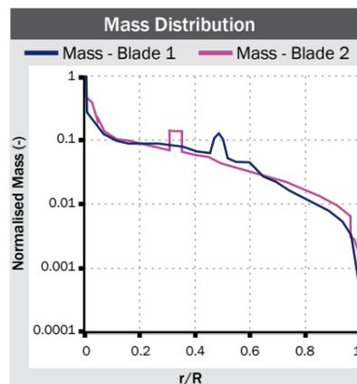
Figure 1: Sectional blade normalised mass distribution.
