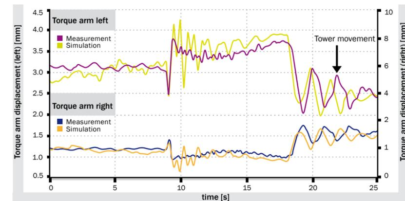
Figure 2: Torque arm displacement - longitudinal.
