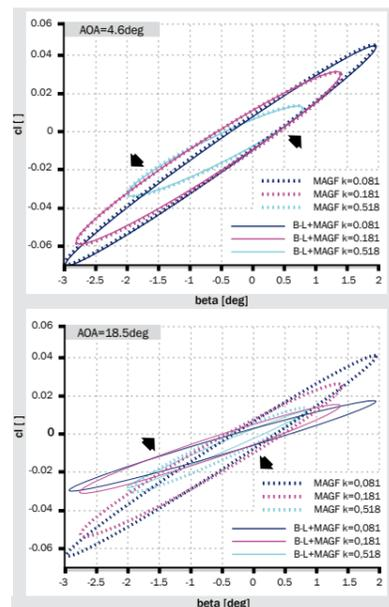
$\Delta$ CL loops as function of  $\beta$  for AOA at 4.60 (left) and 18.50 (right). The trailing edge deflection  $\beta$  ranges from -30 to 1.970 for reduced frequency  $k=\omega c/(2U_0)=0.081$ , for  $\beta=-2.80$  to 1.30 the  $k=\omega c/(2U_0)=0.181$  and finally for  $\beta=-20$  to 0.760 the  $k=\omega c/(2U_0)=0.518$ . Arrows indicate the orientation of the loops in time.
