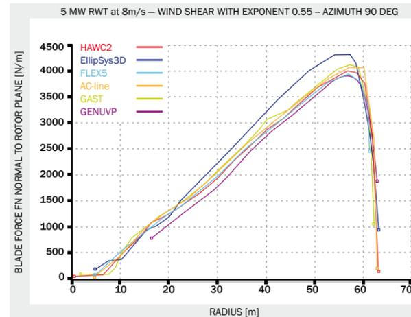
Figure 2b: Predicted blade axial force at 90 and 270 degrees azimuth by different models
