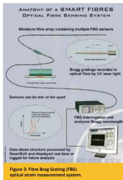
Figure 3: Fibre Brag Grating (FBG) optical strain measurement system.
