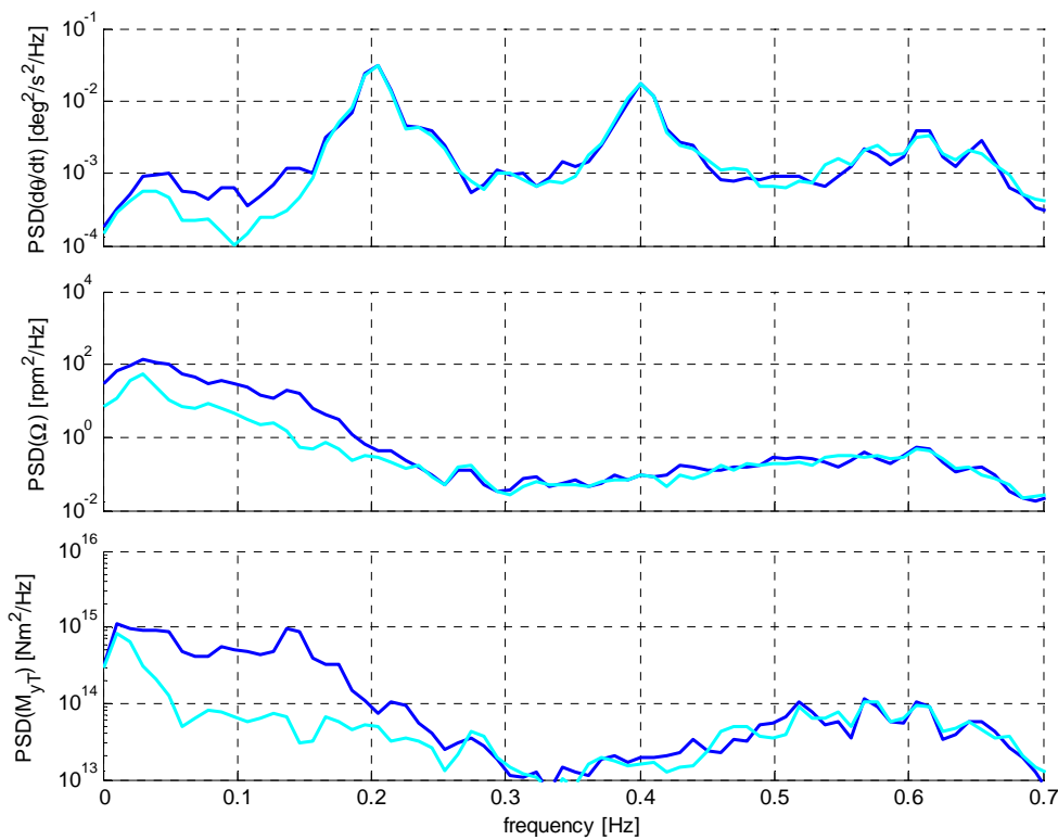
Figure 10: Power spectral density of pitch rate, rotor speed and tower base fore-aft bending moment for a simulation with 16 m/s, UpWind controller only (dark blue) and with feedforward and prediction time \tau_{Sim} (light blue).
