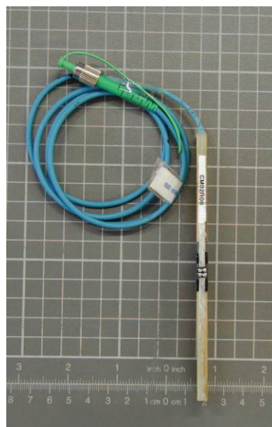
Figure 8: Side view of reference geometry specimen with embedded fibre
