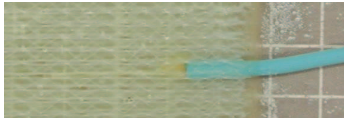
Figure 7: Embedded sensor before applying specimen tabs
