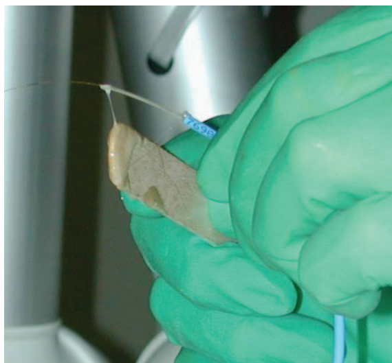
Figure 3: Sealing mantle with Araldite
