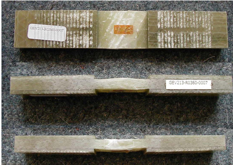
Figure 44: Front & Lateral side of a failed [60] 7 coupon in compression
