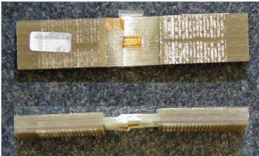
Fig. 48: Failed [0]_4 coupon in compression
