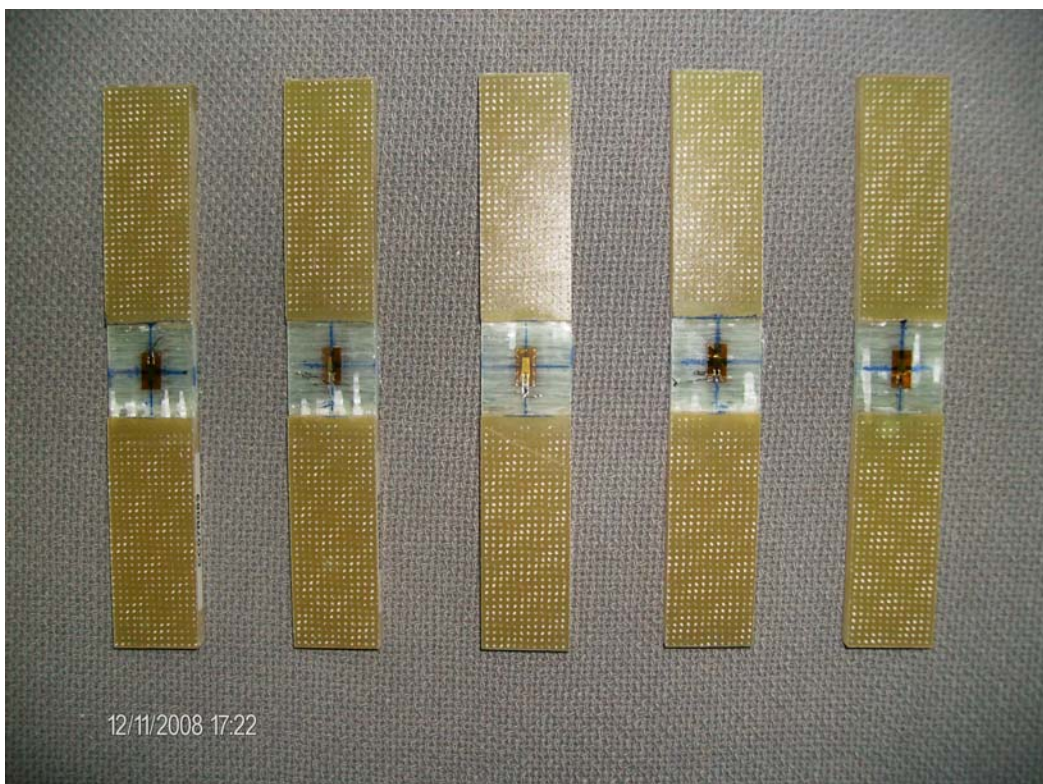
Fig. 75: Photo of the tested coupons CC07R089, CC08R089, CC11R089, CC12R089 and CC03R089 (from left to right)
