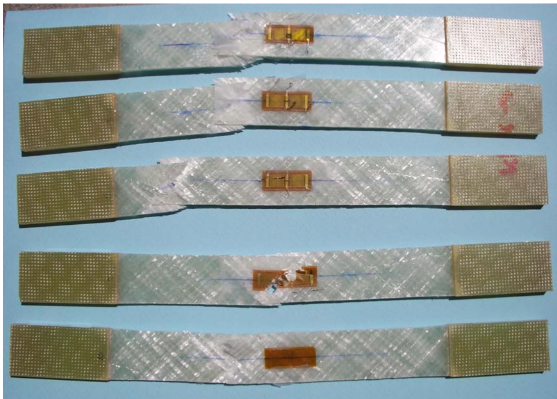
Fig. 153 Photo of failed coupons KJ10I10 to KK04I10 (bottom-up)
