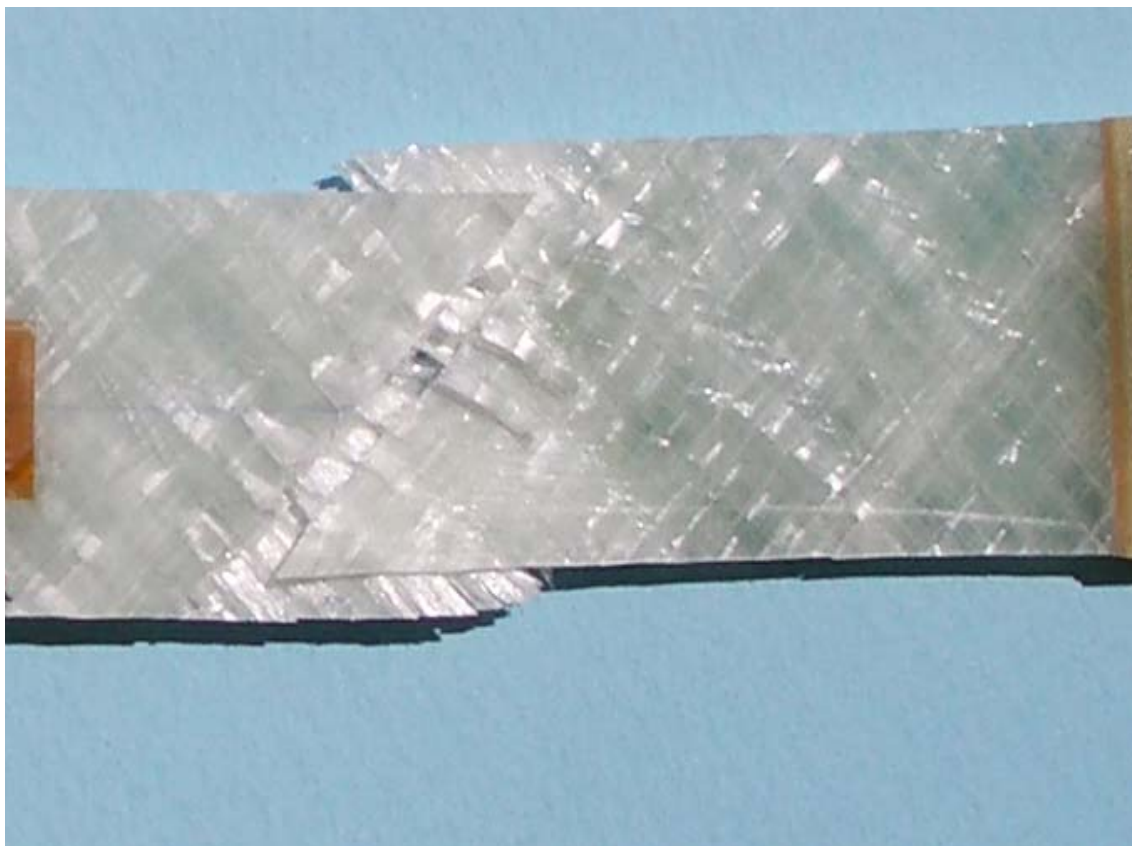
Fig. 155 Detail of failed coupon KK05110
