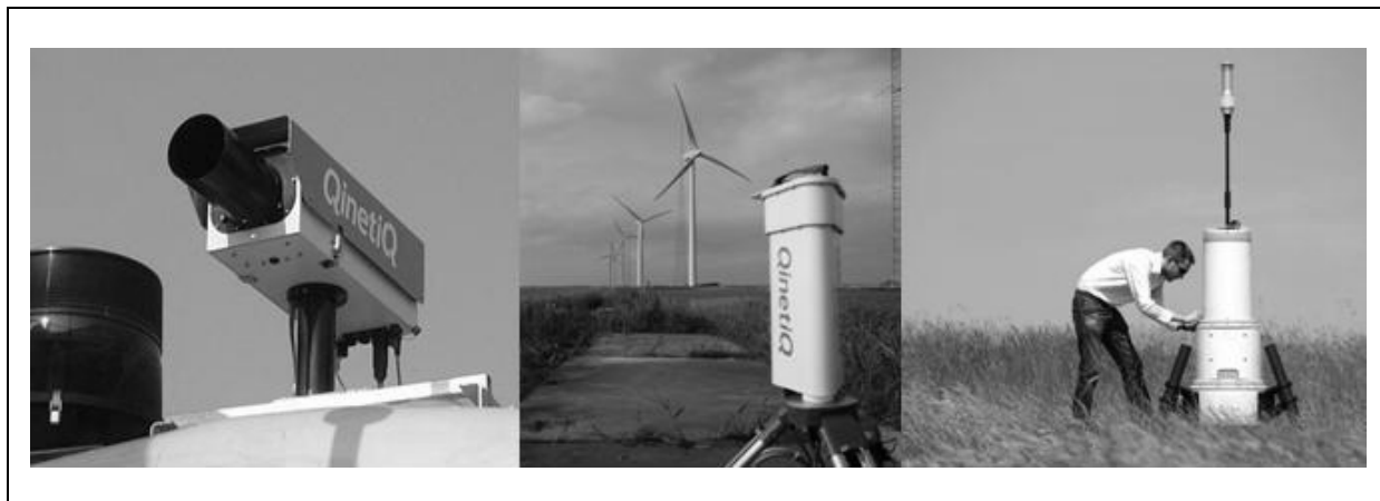
Figure 3: Evolution of the ZephIR lidar. The left-hand picture 3a shows the lidar head mounted on the nacelle of a Nordex N-90 wind turbine. The central picture 3b shows a prototype ground-based wind profiler at Risø wind energy test site, Høvsøre, Denmark. The right-hand picture 3c shows the ZephIR production model deployed in the field.
