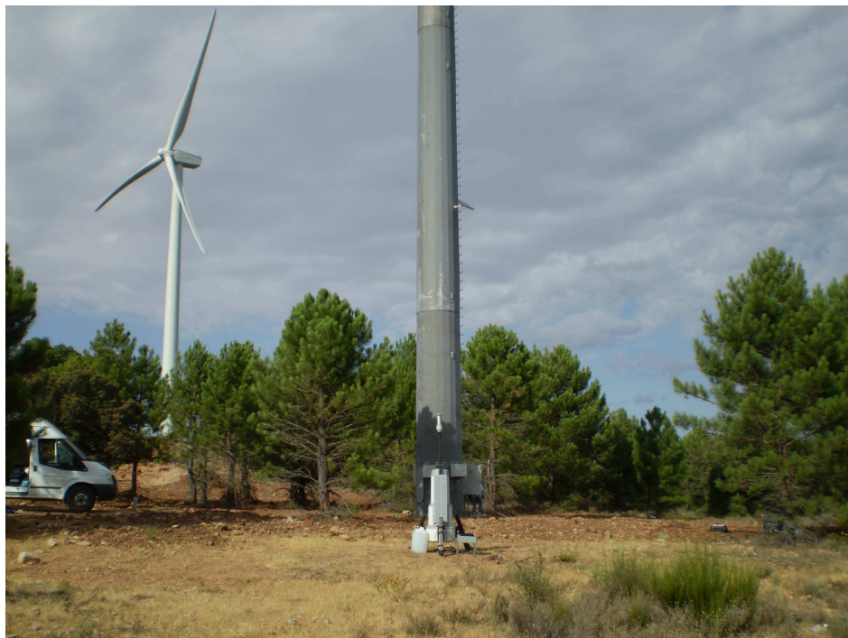
Figure 5: Position of lidar relative to reference mast and wind turbine under test.
