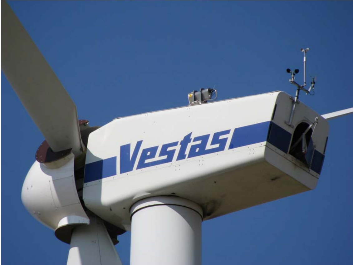
Figure 5 The Risø V27 wind turbine with the ZephIR prototype CW lidar mounted on the top of the nacelle.
