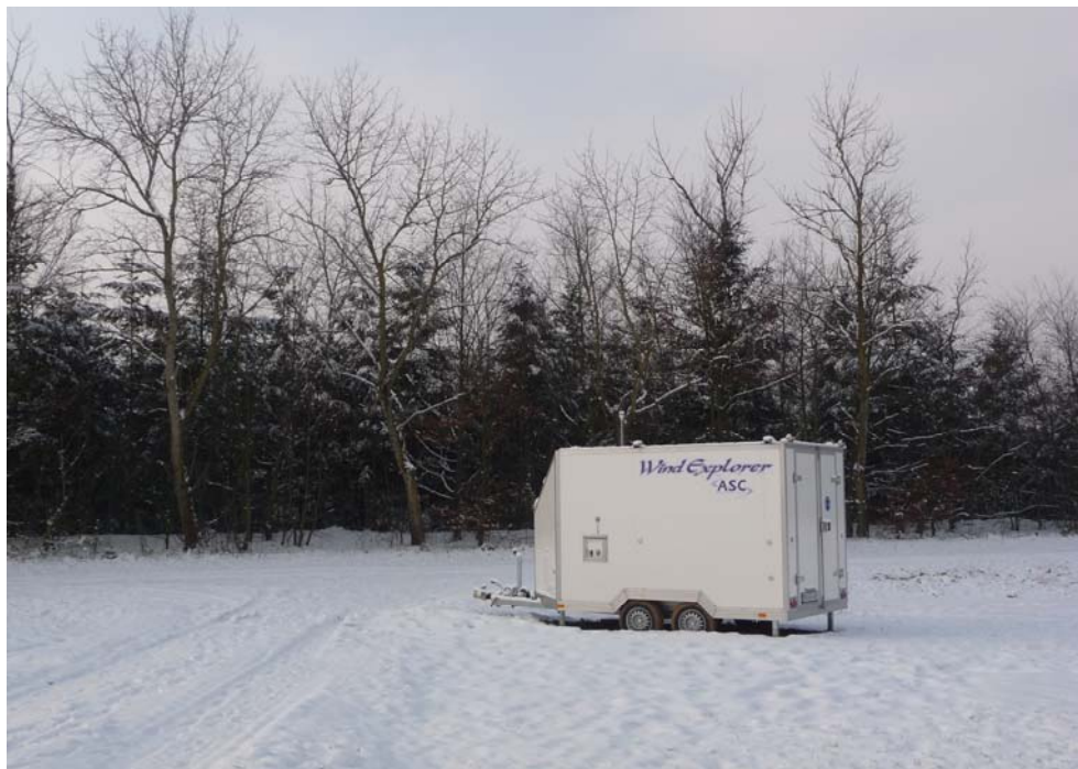
Figure 3.7.5 – ASC4000 Wind Explorer SODAR set-up at Wind Test Grevenbroich's turbine
