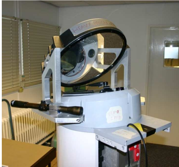
Figure 1: Mirror clamped at 45-degree angle to the ZephIR optics pod for focus calibration.
