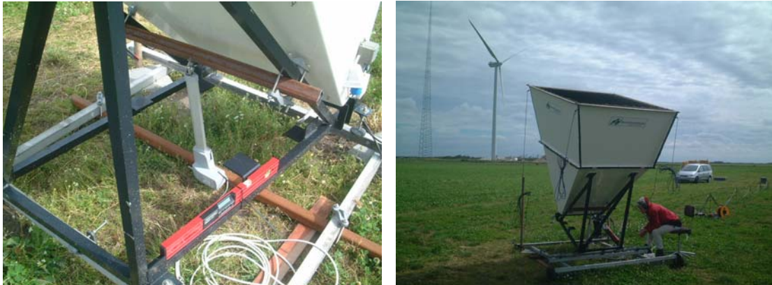
Figure 3. The mounting frame and linear actuator, with digital level (left photograph) and measurements being taken (right photograph).
