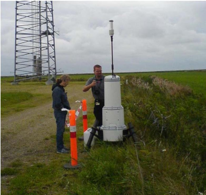
**Figure 3 A ZephiR lidar on test 40m from the meteorological mast.**
