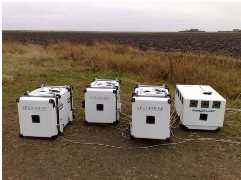
**Figure 4 Four Leosphere Windcubes on simultaneous test at the base of the meteorological mast.**
