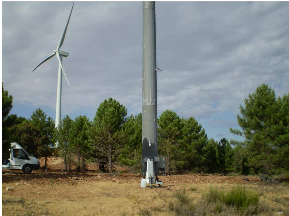
**Figure 4:** Position of lidar relative to mast and wind turbine.
