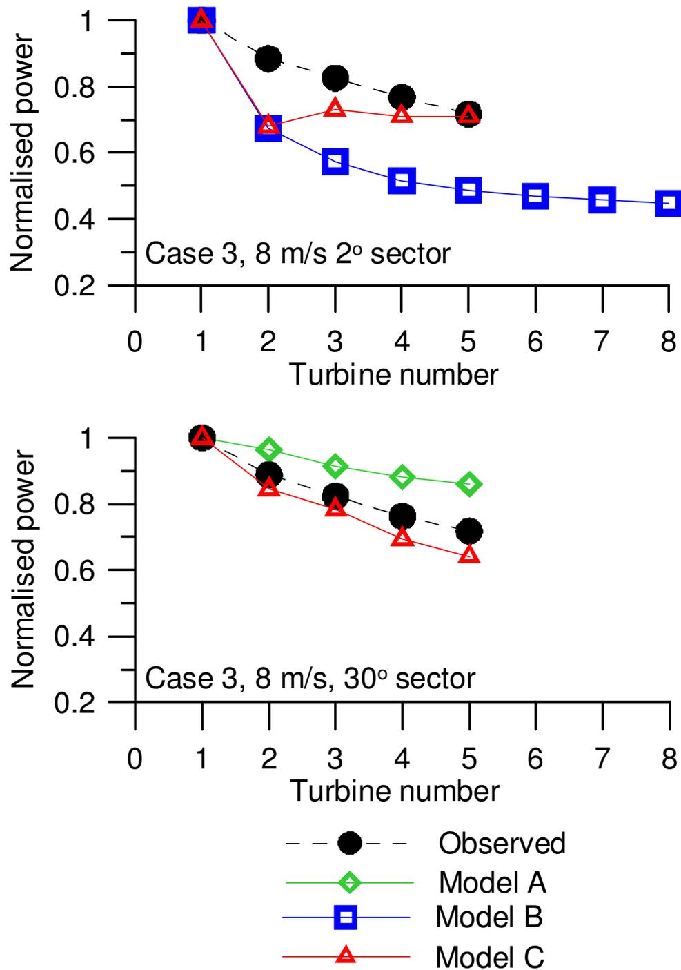
Figure 9: Preliminary comparison of models and measurements for three wind speed scenarios at Horns Rev (direction 345°, case 3 in Figure 4). (Continued).
