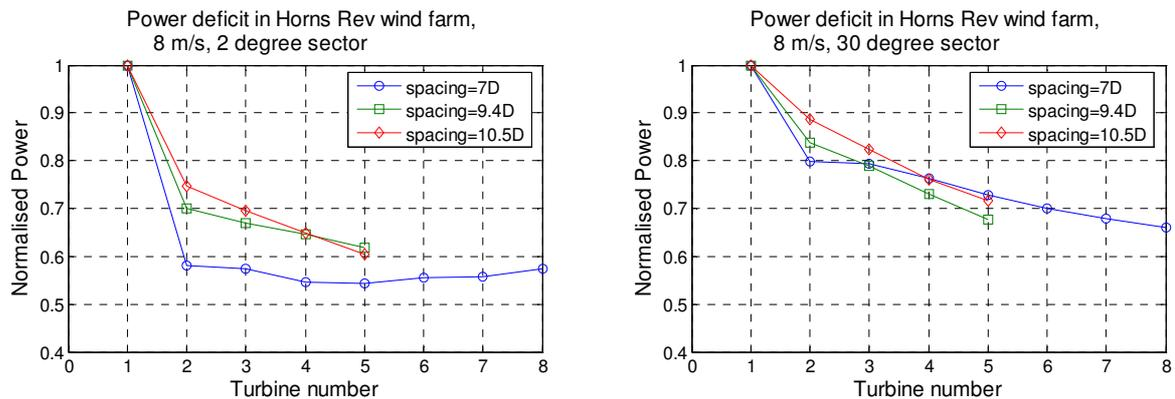
Figure 5: Power deficit inside Horns Rev wind farm for  $V=8\pm 0.5$  m/s inflow for different spacing.
