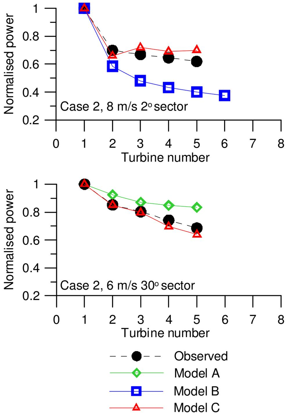
Figure 8: Preliminary comparison of models and measurements for three wind speed scenarios at Horns Rev (direction 315°, case 2 in Figure 4). (Continued).
