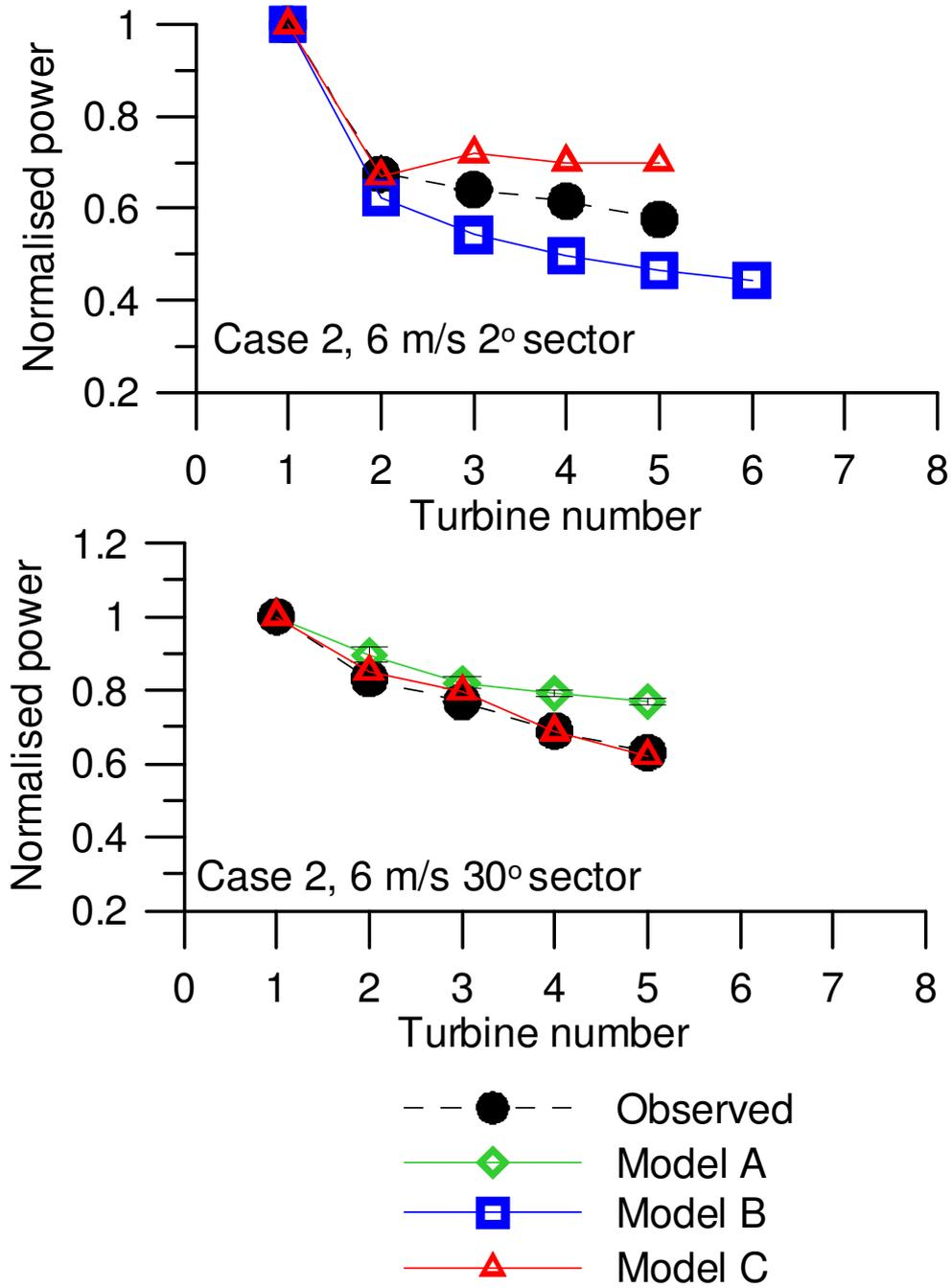
Figure 8: Preliminary comparison of models and measurements for three wind speed scenarios at Horns Rev (direction 315°, case 2 in Figure 4). (Continued).
