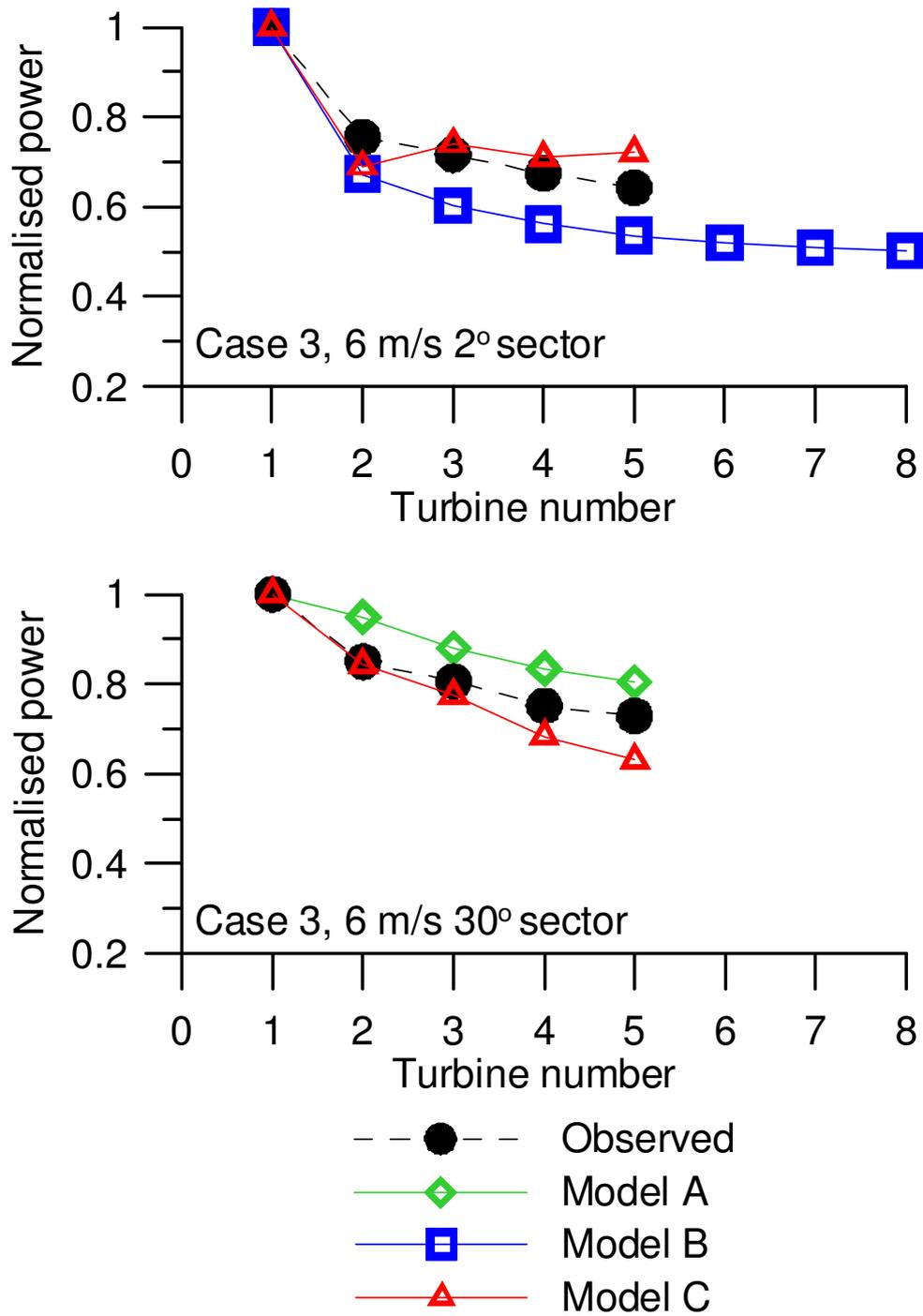
Figure 9: Preliminary comparison of models and measurements for three wind speed scenarios at Horns Rev (direction 345°, case 3 in Figure 4).
