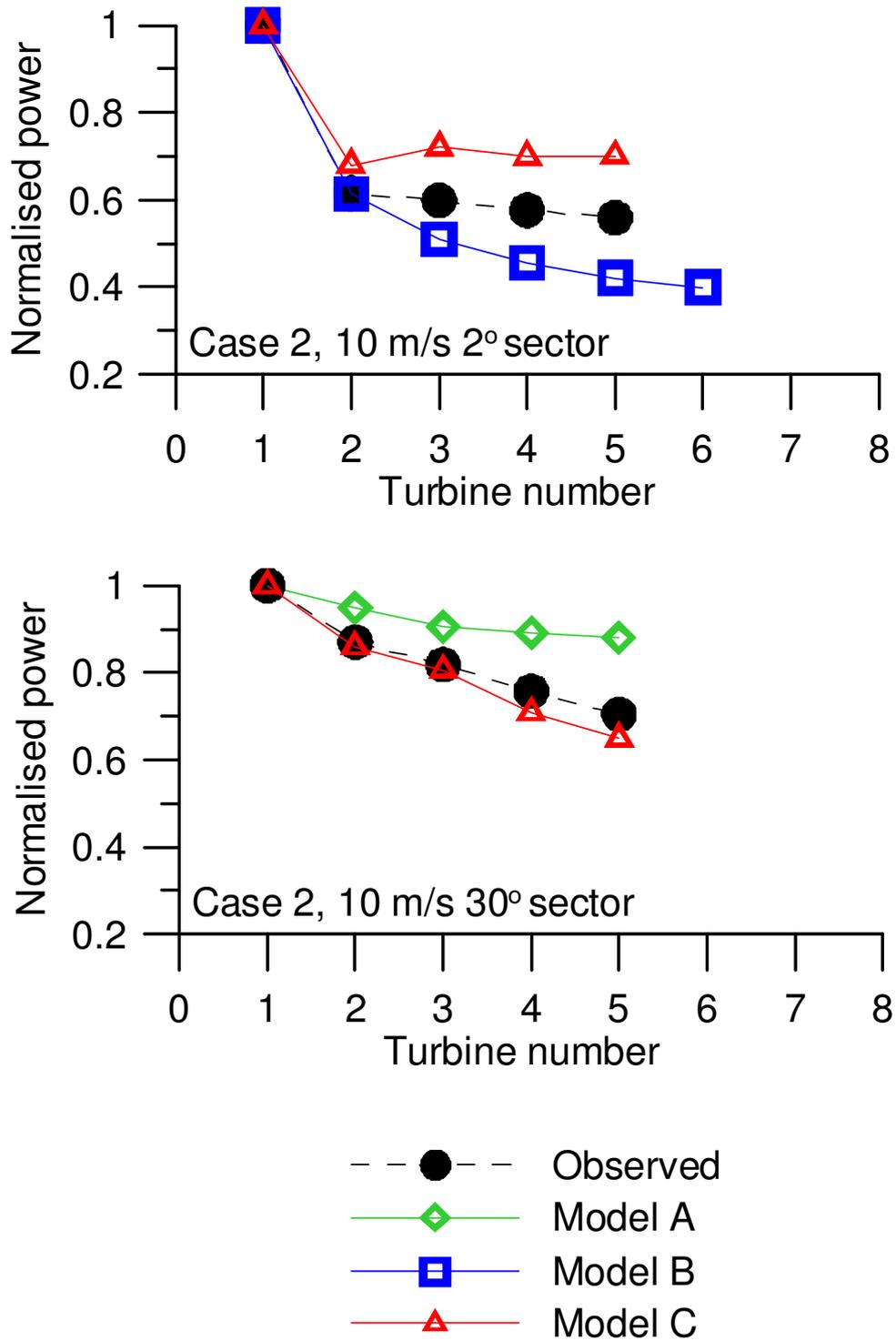
Figure 8: Preliminary comparison of models and measurements for three wind speed scenarios at Horns Rev (direction 315°, case 2 in Figure 4). (Continued).
