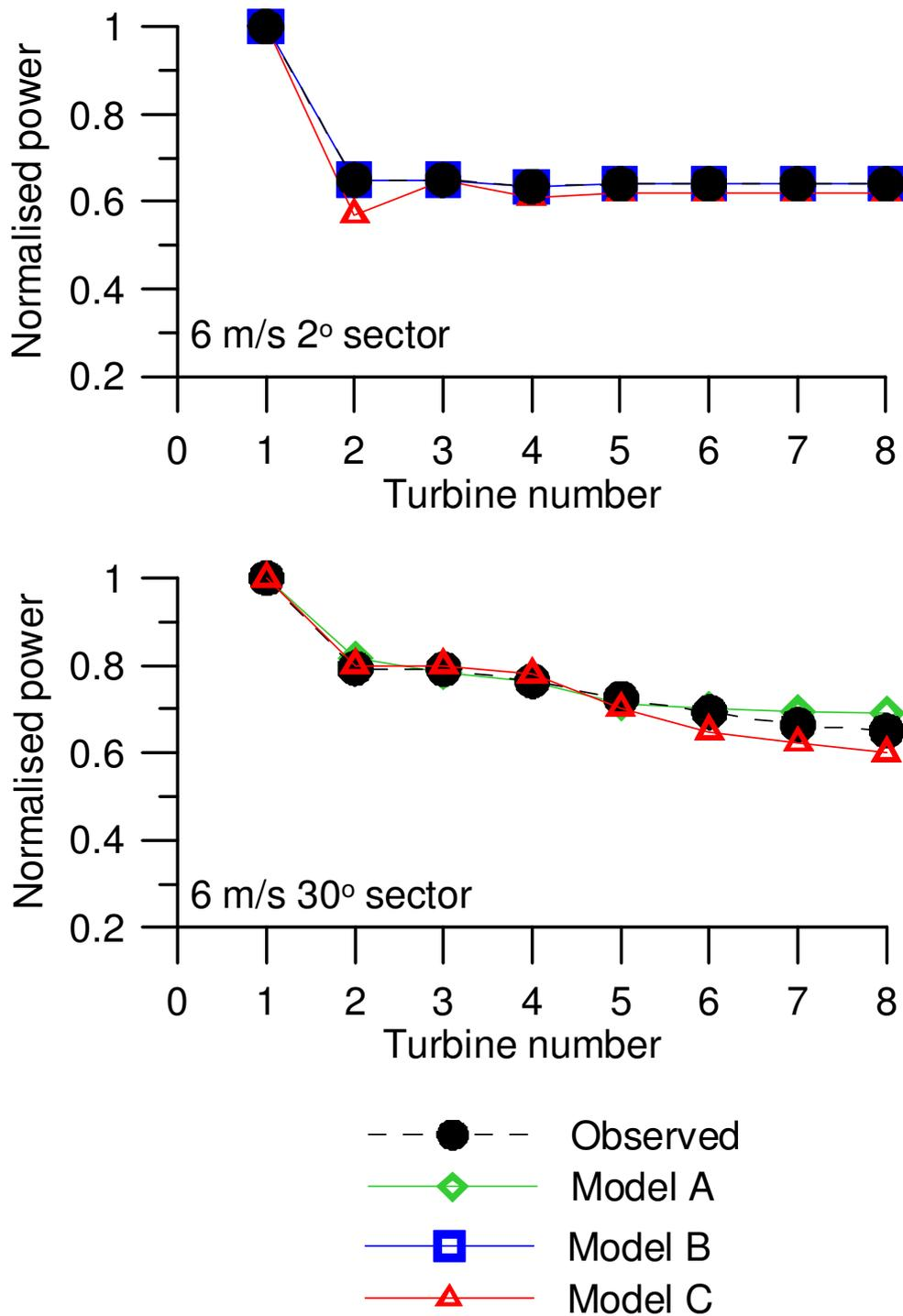
Figure 7: Preliminary comparison of models and measurements for three wind speed scenarios at Horns Rev (direction 270°, case 1 in Figure 4).
