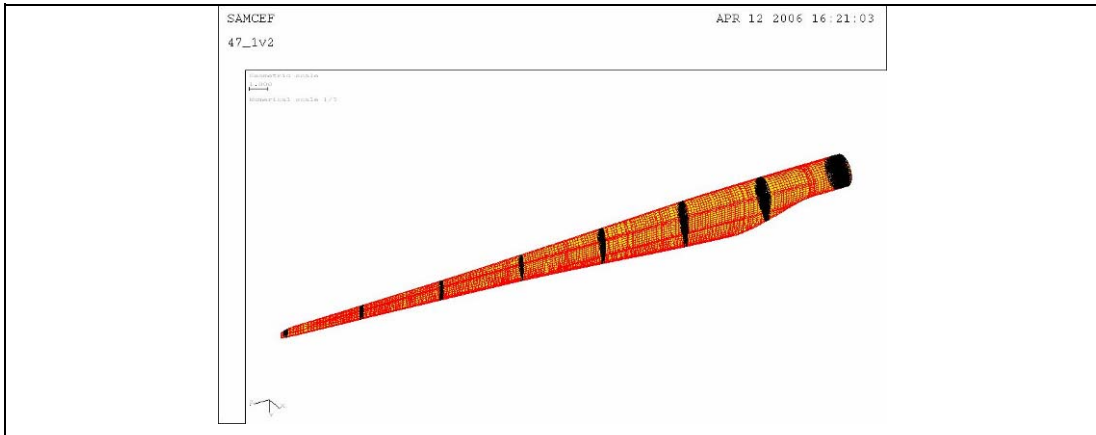
Figure 3a: FEM Model blades: anisotropic multiplayer shell composite elements. Condensed to Super Element
