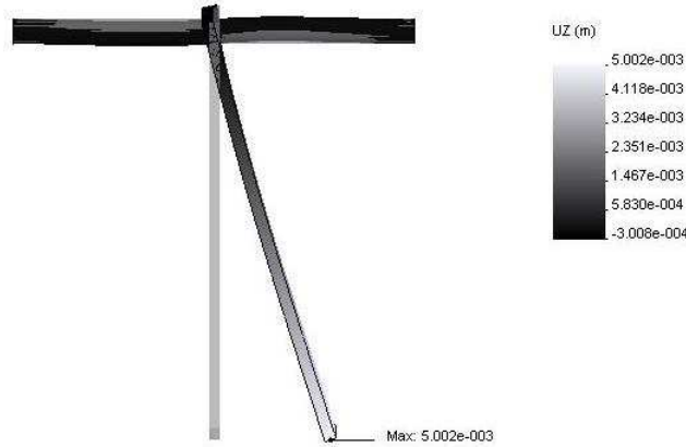
Fig. 22(a) One thirtieth finite element model of stator disc and beam support showing deflection when R=5.34\text{mm}
