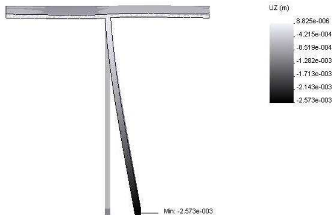
Fig. 22(b) One thirtieth finite element model of stator disc and cylindrical casing showing deflection when t_c=3.13\text{mm}
