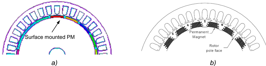
Fig. 2-5: Basic configurations of RFPM machines with surface mounted (a) and flux concentrating (b)
