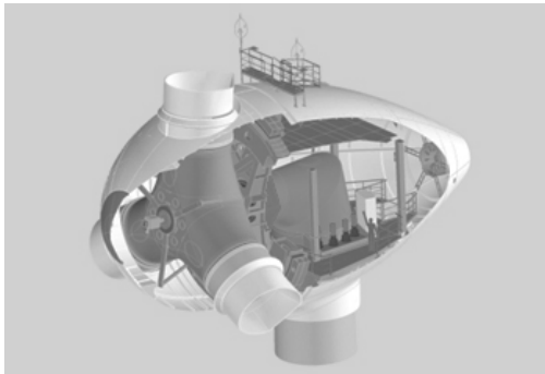
Figure 1: Structure of 4.5 MW EESG DD. Source: Enercon GmbH [7]
