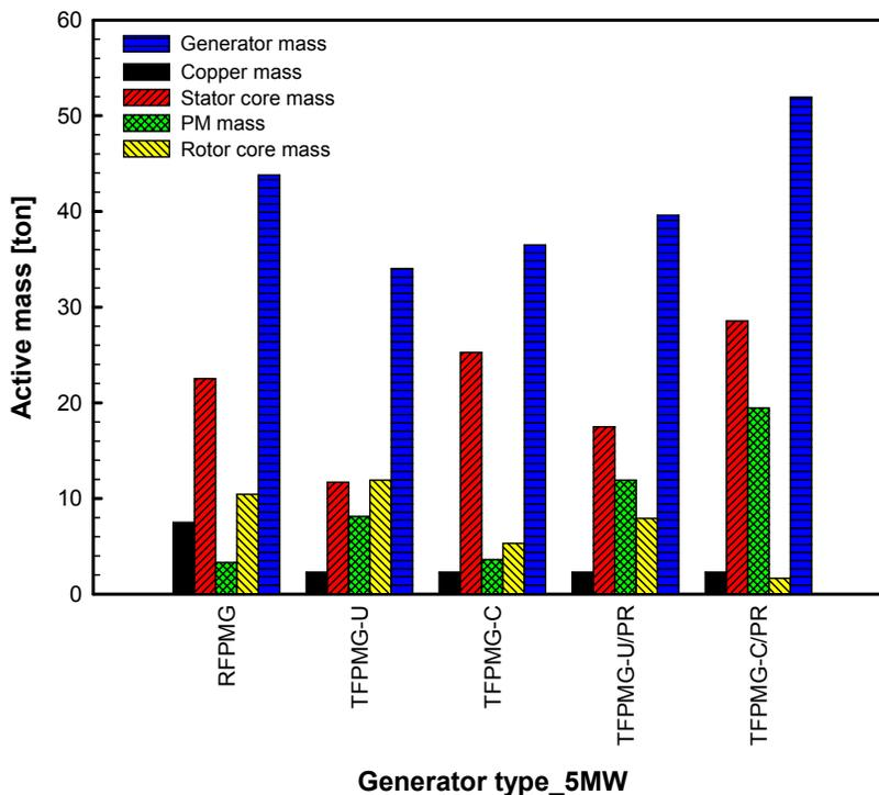
Figure 2-13: Active mass comparison of different 5 MW PM generators
