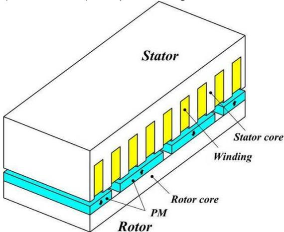
**Figure 2-1:** Surface-mounted RFPM generator (RFPMG)
