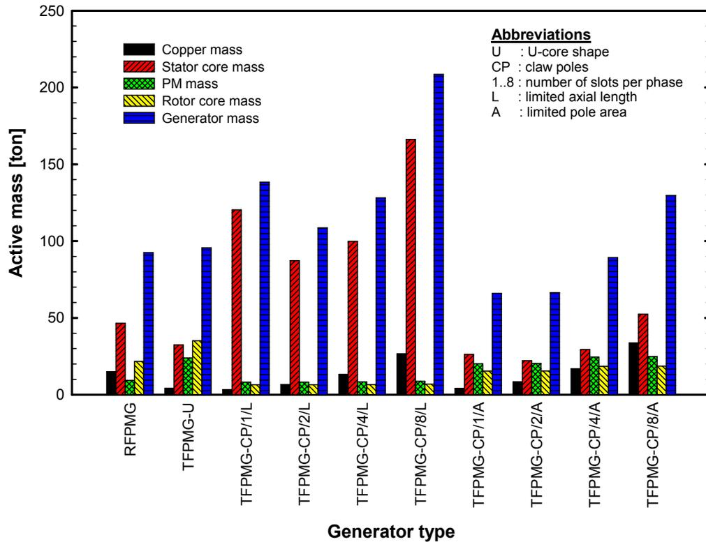
Figure 3-20: Active mass of different PM generators for 10 MW direct-drive wind turbines
