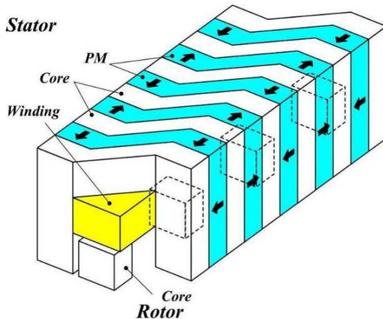
**Figure 2-5:** Double-sided single winding flux-concentrating TFPM generator with a C-core (TFPMG-C/PR)
