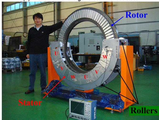
(c) Generator with rotor and stator
