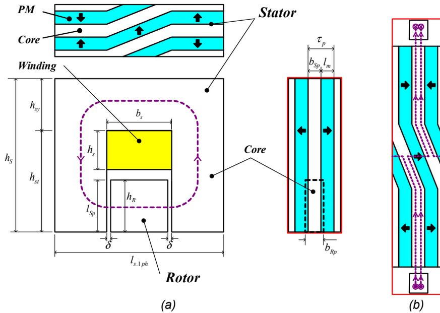
Figure 2-10: Dimensional parameters and flux paths of TFPMG-C/PR
