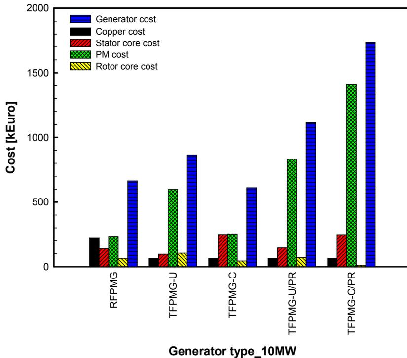
**Figure 2-18:** Cost comparison of different 10 MW PM generators
