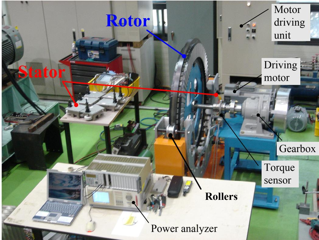
Figure 3-12: Proposed TFPM generator with experimental setup
