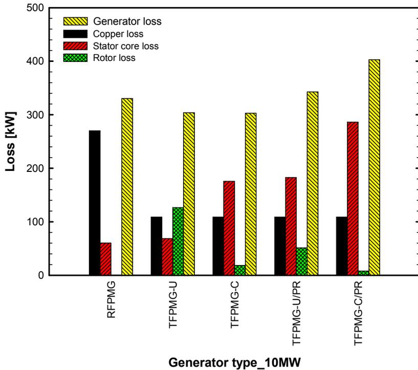
Figure 2-17: Loss comparison of different 10 MW PM generators
