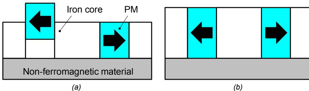
**Figure 3-1:** Conventional PMs and iron cores configuration of the flux-concentrating TFPM machine
