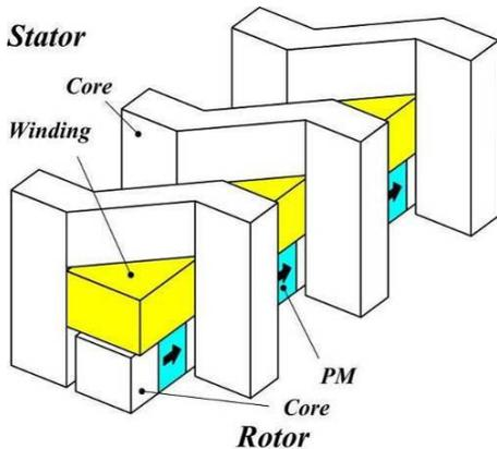
**Figure 2-3:** Double-sided single winding flux-concentrating TFPM generator with a C-core (TFPMG-C)
