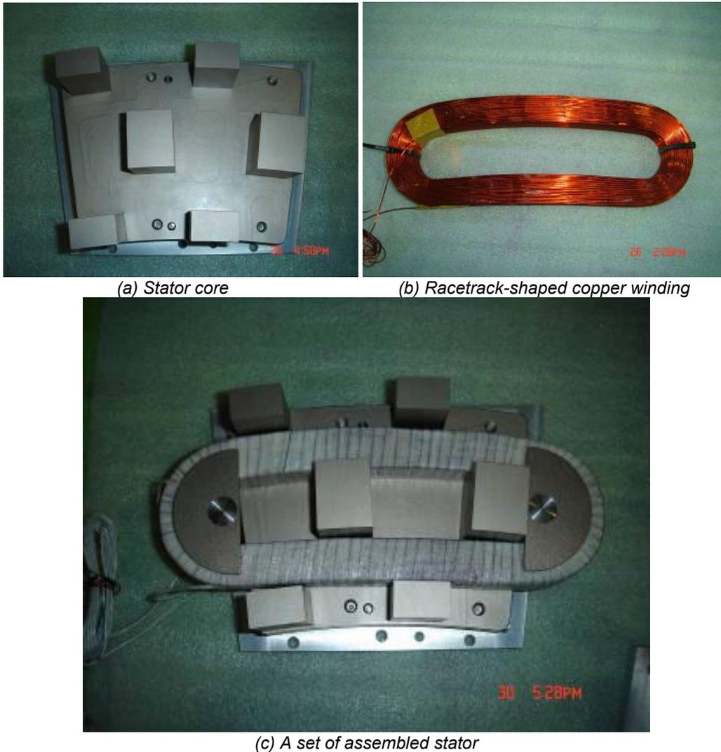
**Figure 3-10:** The set of stator cores and racetrack-shaped winding of the proposed TFPM generator (supported by Wintech Co., Ltd. in Korea)
