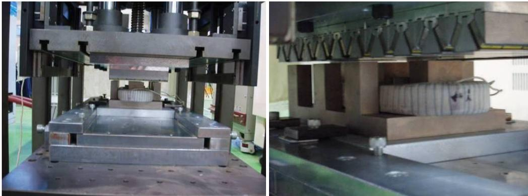
Figure 3-14: Proposed TFPM generator equipped on a test bench to measure the static force
