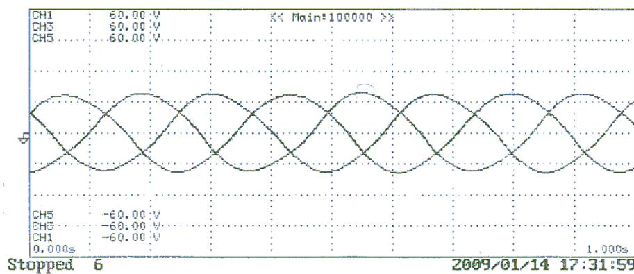
Figure 3-13: No-load induced voltages measured at 0.25 m/s
