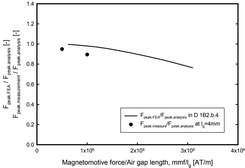
Figure 3-16: Thrust force differences between the measurement and the analysis
