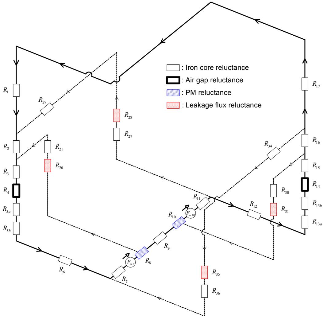
**Figure 3-7:** Equivalent circuit of magnetic reluctances of the proposed TFPM generator
