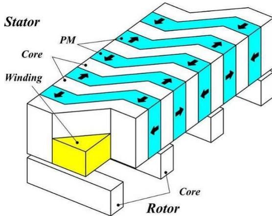
**Figure 2-4:** Single-sided single winding flux-concentrating TFPM generator with a U-core (TFPMG-U/PR)
