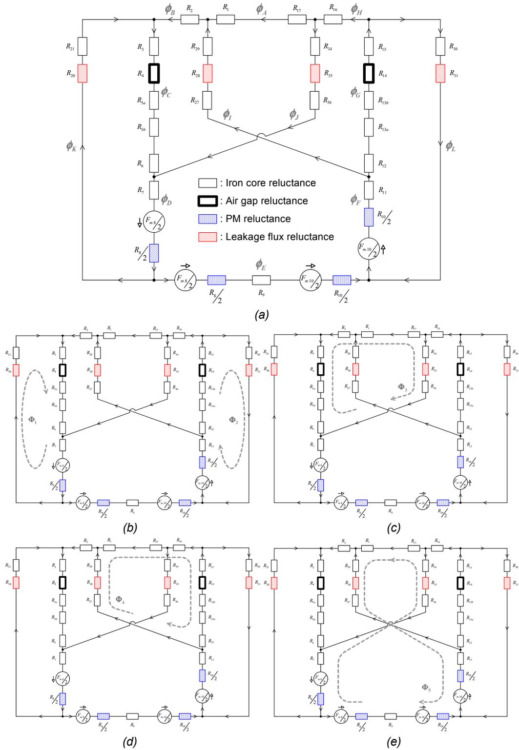
**Figure 3-8: Modified equivalent circuit of magnetic reluctances of the proposed TFPM generator**
