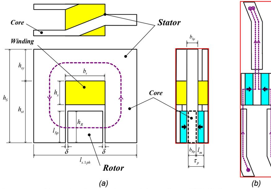
Figure 2-8: Dimensional parameters and flux paths of TFPMG-C
