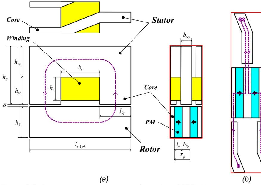
Figure 2-7: Dimensional parameters and flux paths of TFPMG-U
