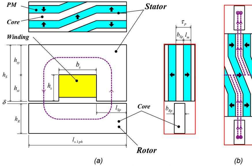
Figure 2-9: Dimensional parameter and flux paths of TFPMG-U/PR
