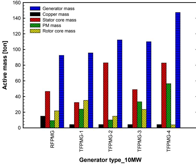
Figure 2-16: Active mass comparison of different 10 MW PM generators
