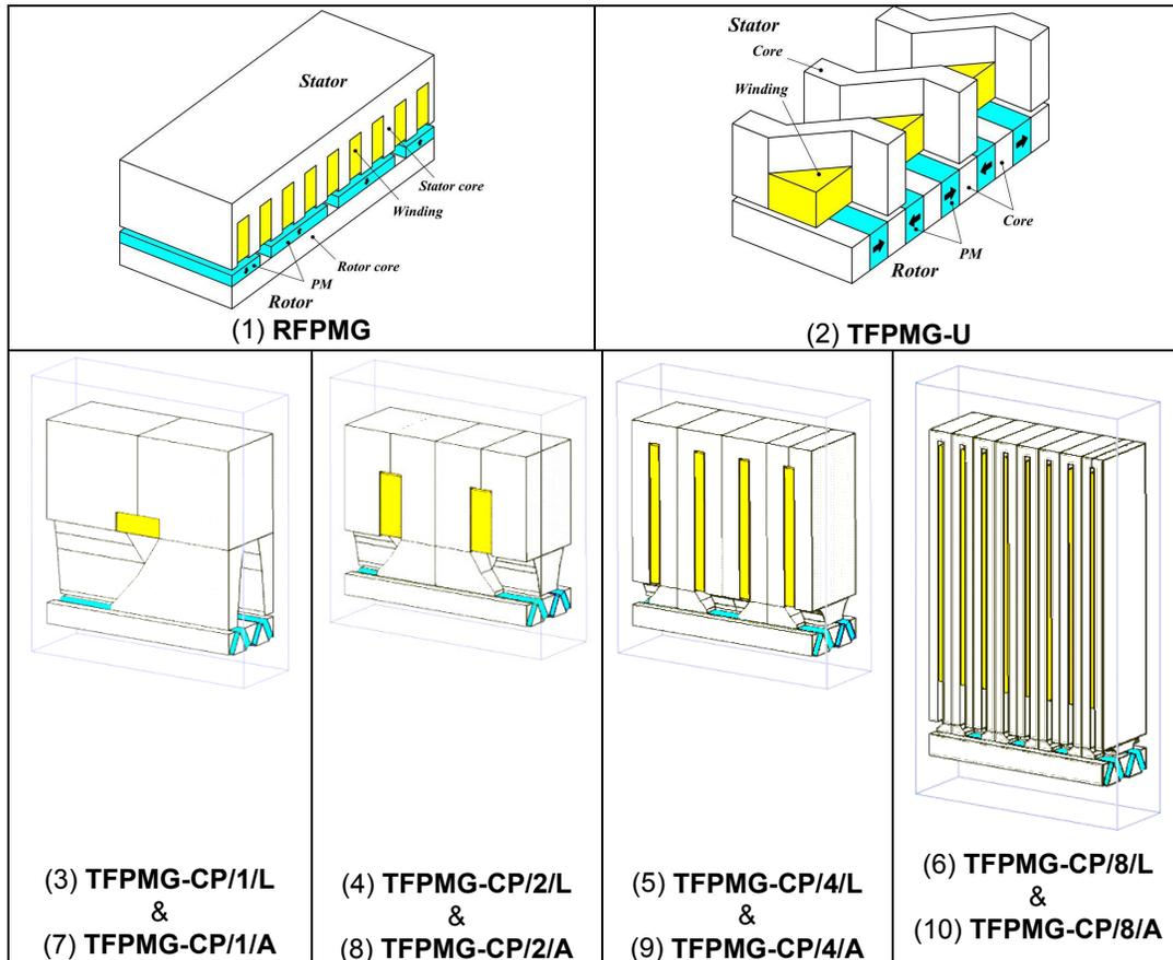
**Figure 3-17: External shapes of the ten PM generators**
