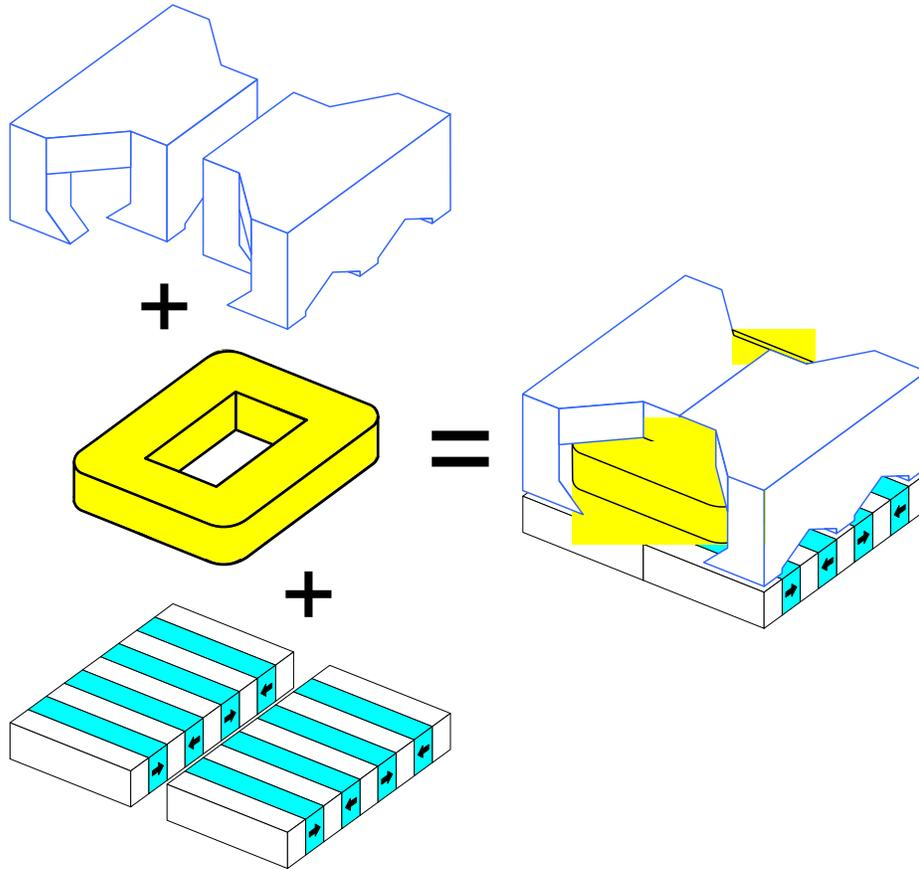
**Figure 3-3:** New TFPM machine with flux-concentrating configuration
