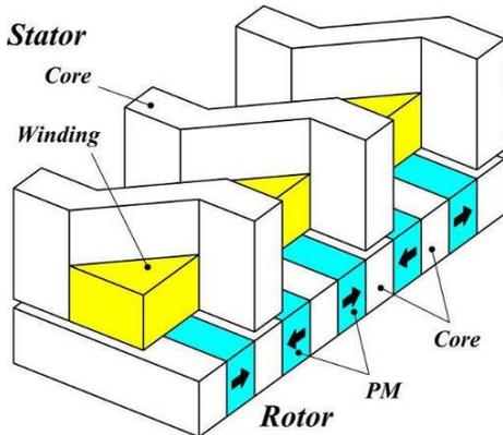
**Figure 2-2:** Single-sided single winding flux-concentrating TFPM generator with a U-core (TFPMG-U)
