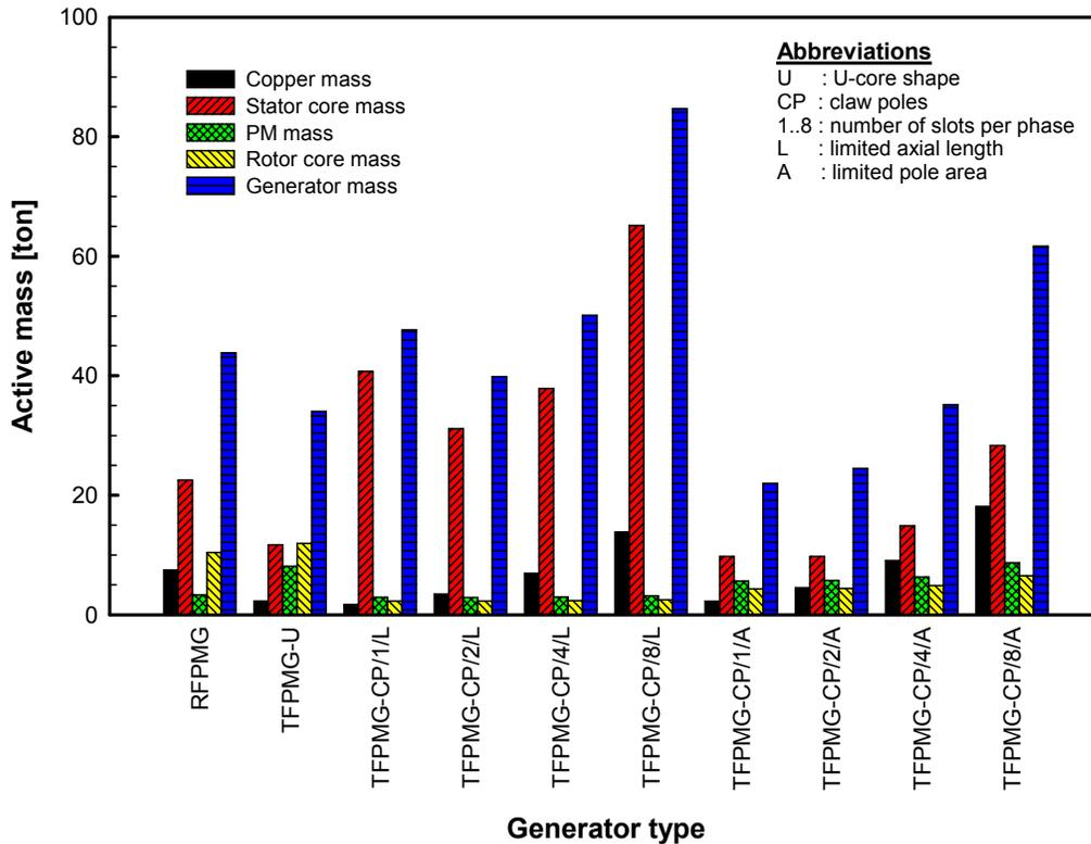
**Figure 3-18:** Active mass of different PM generators for 5 MW direct-drive wind turbines
