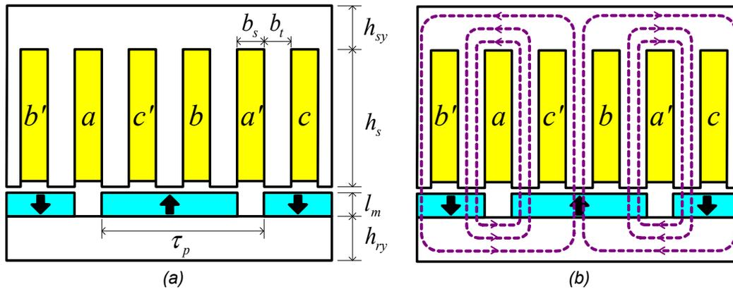
**Figure 2-6:** Dimensional parameters and flux paths of RFPMG
