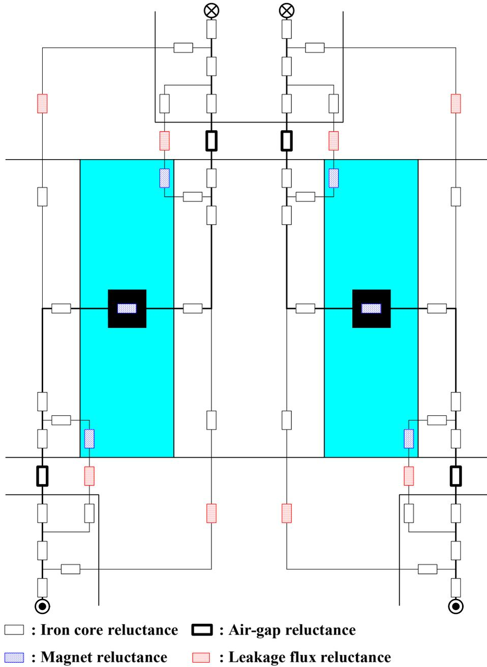
**Figure 2-11:** Equivalent circuits of magnetic reluctances of TFPMG-U and TFPMG-C
