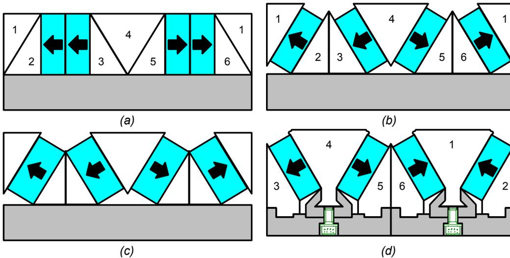
**Figure 3-4:** New PMs and iron cores configuration of the flux-concentrating TFPM machine
