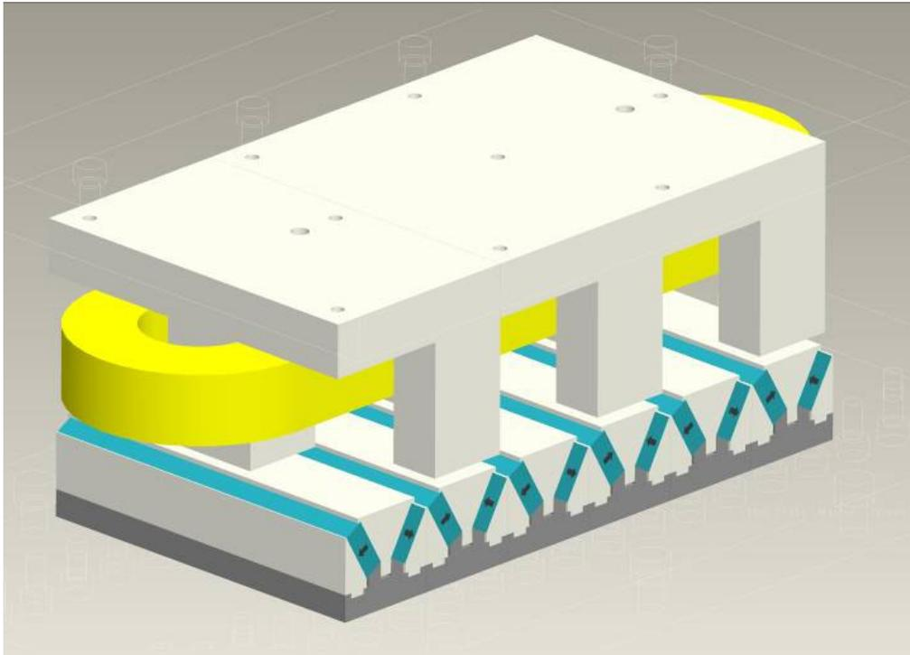
**Figure 3-5:** 3D sketch of multiple-module TFPM generator with two slots per phase
