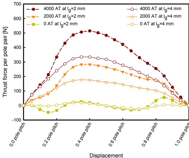
Figure 3-15: Thrust force per a pole pair of the proposed TFPM generator by the measurement
