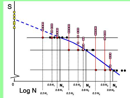
Stress levels for testing the residual strength after a percentage of the expected life
