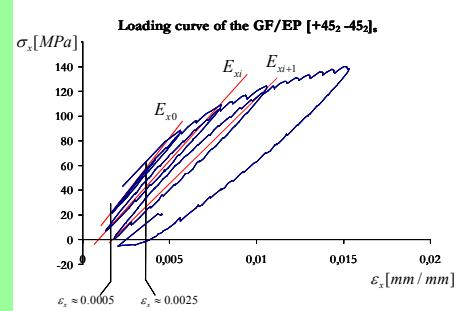
Degradation of Stiffness during Fatigue Life
