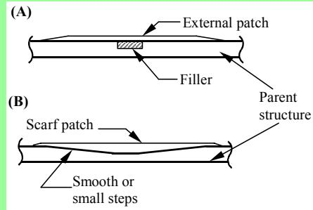
Plug/Patch and scarf repair systems
