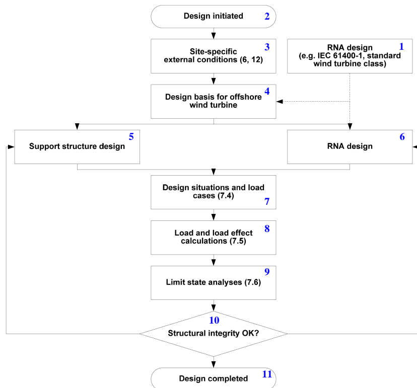
Figure 5.1: Design process for an offshore wind turbine [8]
