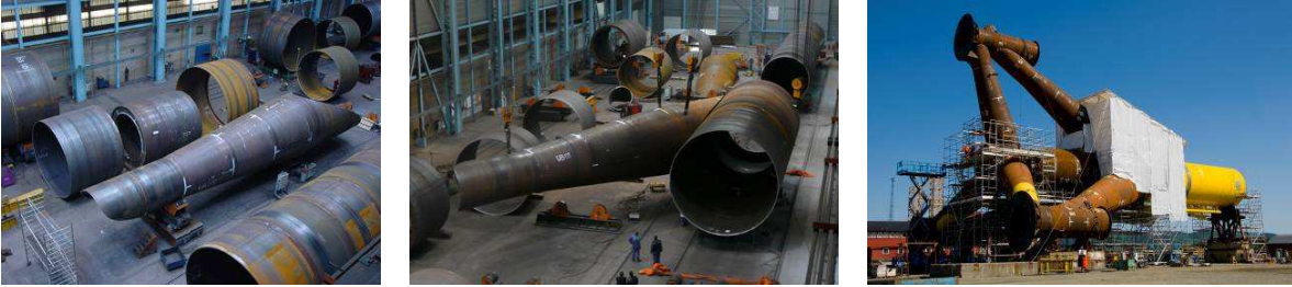
Figure 3.2: Various stages in the manufacturing of a tripod structure [42]
