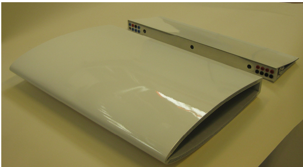
Fig. 30. Adaptive modular airfoil prototype based on R-phase actuated SMA composites
