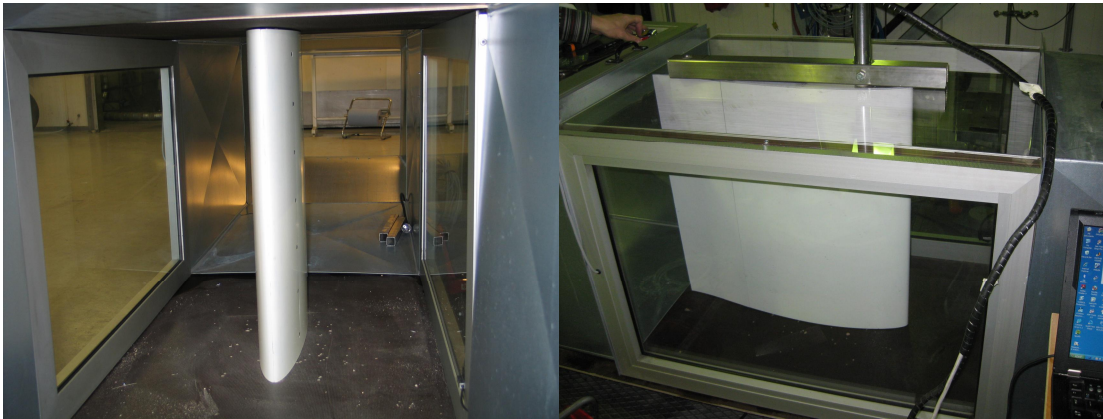
Fig. 33. Wind tunnel test setup.
