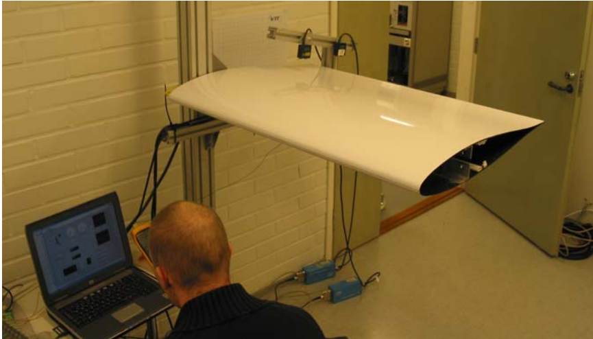
Figure 3: Adaptive airfoil in preliminary testing before installation to the wind tunnel.
