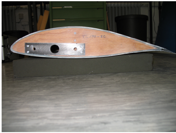
Fig. 7 Side view of the TL 190-82 wind tunnel model
