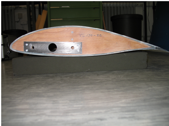
Fig. 6 Flap hinge region of the TL 190-82 wind tunnel model
