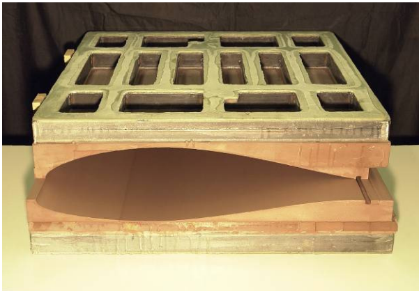
Fig. 1 Negative mold for the NACA wind tunnel model
