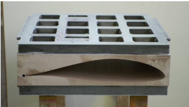
Fig. 5 Negative mold of the TL 190-82 wind tunnel
