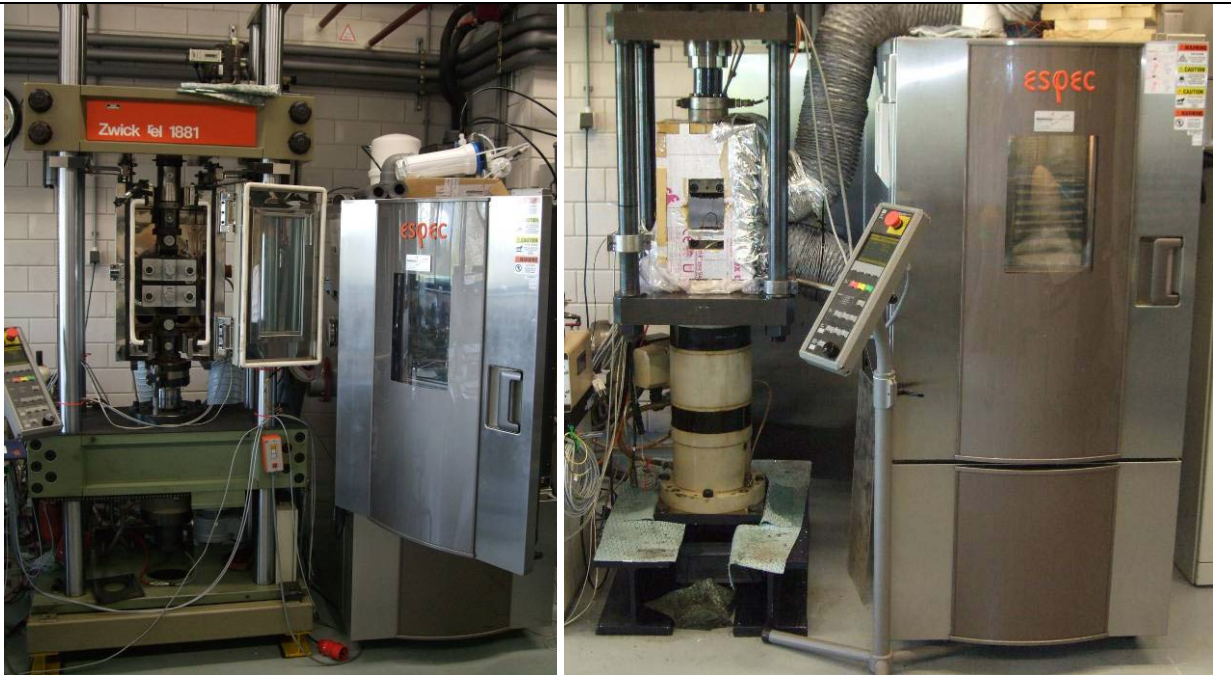
Figure 2: Test set-up using Zwick 220 kN (left) and ZB 100 kN maximum capacity test frames next to Espec external climate chamber
