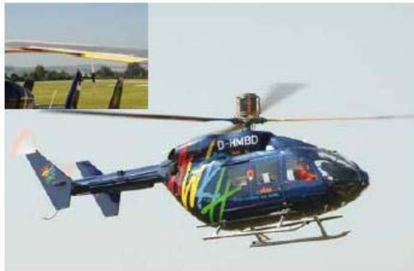
Fig. 21: First flight of a the BK117 S7045 with active trailing edge flaps [10]
