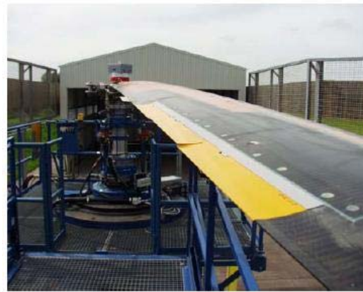
Fig. 18: Blade with flaps on whirl tower
