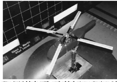
d) Active twist blade with embedded piezoactuators 6-ft-diam rotor test in Glenn L. Martin wind tunnel; produced \pm 0.5 -deg blade twist up to 5/rev excitation
